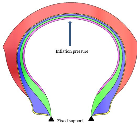
**Fig. 3. Boundary conditions applied on both tyre models.**
