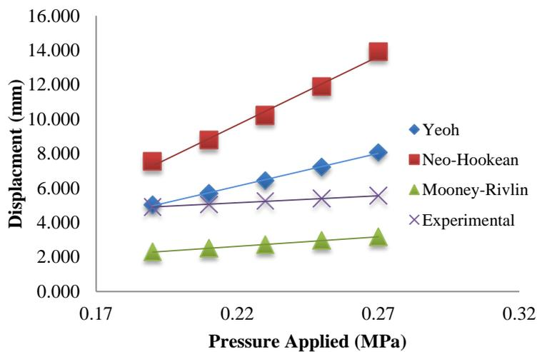
Fig. 8. Comparison of displacement with various material models for single layer tyre model.
