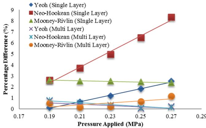
**Fig. 10. Comparison of error percentage with various material models for both tyre models.**
