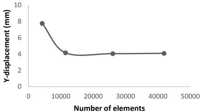
**Fig. 5. Convergence study for mesh discretization.**
