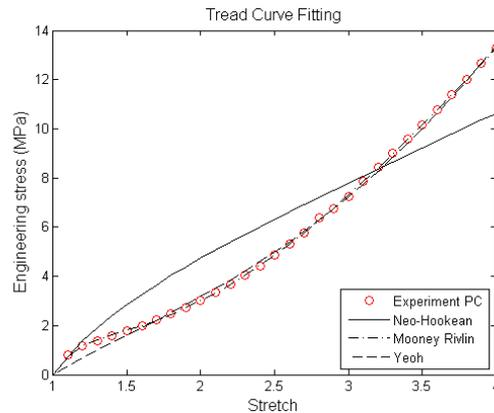
**Fig. 6. Comparison of stress-strain response from uniaxial tensile testing and prediction from material models.**
