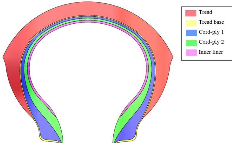
Fig. 2. Multi-layer tyre model.
