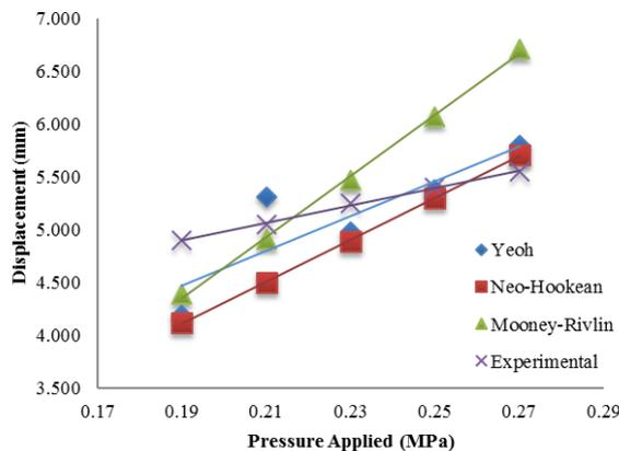
**Fig. 9. Comparison of displacement with various material models for multi-layer tyre model.**
