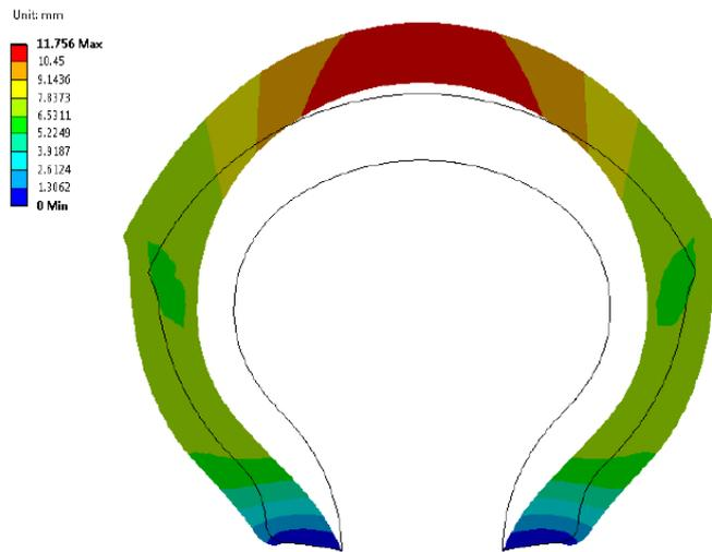
Fig. 7. Tyre model before and after deformation.
