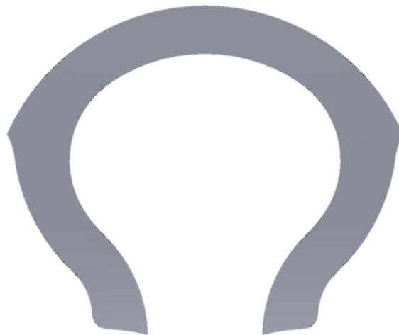
**Fig. 1. Single-layer tyre model based on 80/90-17 bias-ply tyre.**
