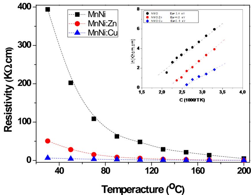
**Figure 4.** Resistivity curves as a function of temperature of NMO ceramics sintered at 1000 °C for 3 h
