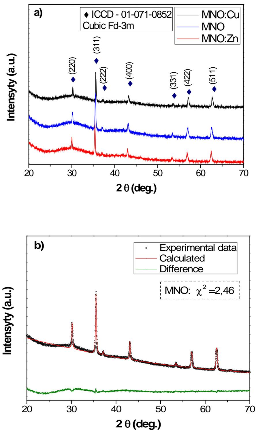
Figure 2. (a) XRD patterns of the  $\text{NiMn}_2\text{O}_4$  ceramics and (b) graphic example of Rietveld fit.
