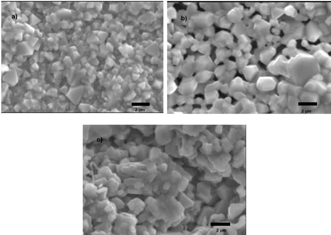
**Figure 3.** SEM images of ceramic  $\text{NiMn}_2\text{O}_4$  (scale 2  $\mu\text{m}$ ). (a) NMO, (b) NMO: Cu, and (c) NMO: Zn
