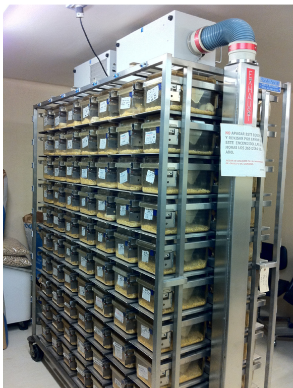
Figure 2: Microisolator system. This equipment consists of 2 parallel racks with several acrylic cages connected to a closed airflow system. The system permits a constant flow of clean air to infected animals and prevents the exit of bacteria from the cages. It can house 1000 infected animals and poses no infection risk to the personnel. The microisolator system is a part of the BSL-3 facilities of the animal house in the National Institute of Medical Sciences, Mexico City.
