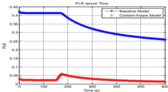
Figure 7: Packet loss ratio against time for downlink video delivery
