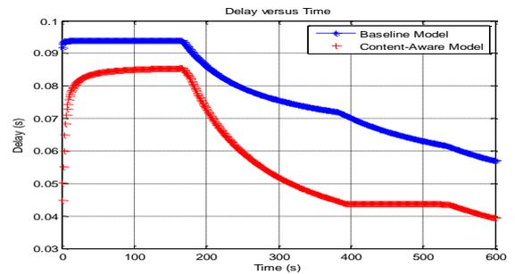
Figure 6: Average delay against time for uplink video delivery
