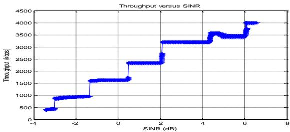
Figure 3: Throughput against SINR plot for downlink transmission (R = 4 Mbps)
