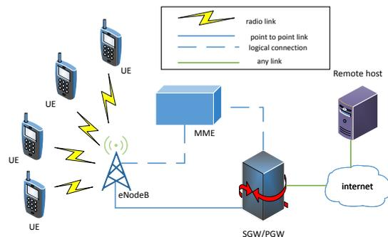
Figure 1: Single eNodeB LTE – EPC simulation topology
