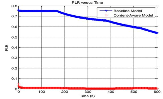
Figure 5: Packet loss ratio against time for uplink video delivery
