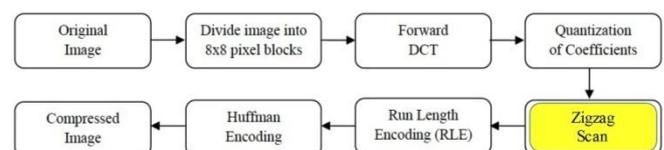
Figure 1: Design of JPEG compression with efficient zigzag scan part [4]
