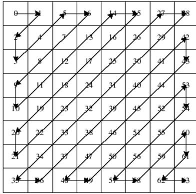
Figure 2: Zigzag scan process on 8 x 8 picture [1]
