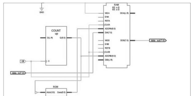
Figure 8: Zigzag scan schematic using the mapping method
