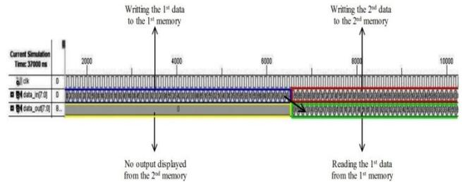
Figure 7: Result from post-route simulation of zigzag scan with mapping process
