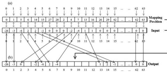
Figure 3: Diagram of zigzag scan with mapping method.
