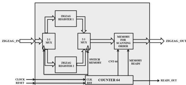
Figure 4: Architecture of zigzag scan [5]
