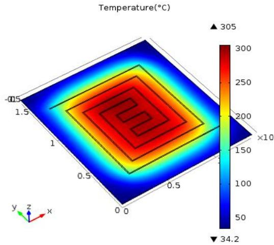
Figure 3: Temperature distribution in a combinative meander-spiral platinum heater
