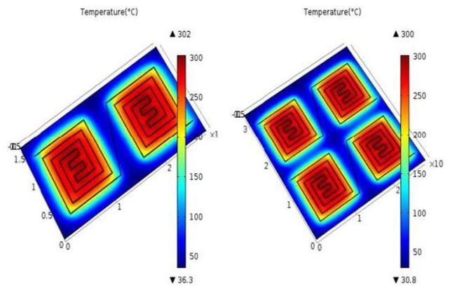
Figure 6: Thermal distribution for platinum multi-sensor.
