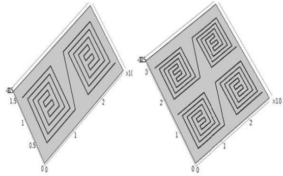
Figure 5: Multi-sensor (a) two and (b) four chips.
