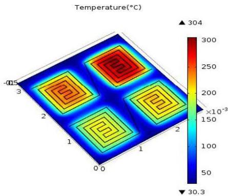
Figure 8: Different detection temperatures for the multi-sensor.
