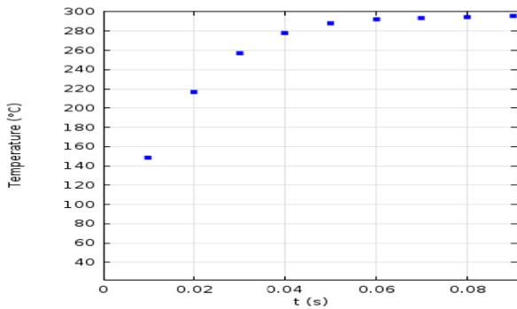
Figure 4: Temperature temporal variations along the horizontal axis to the surface of the heating platform for a combinative meander-spiral heater
