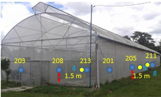
Figure 1: Diagram showing greenhouse with node position side view
