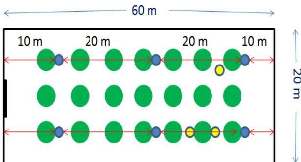
Figure 2: Diagram showing nodes position among the vegetation in greenhouse from top view
