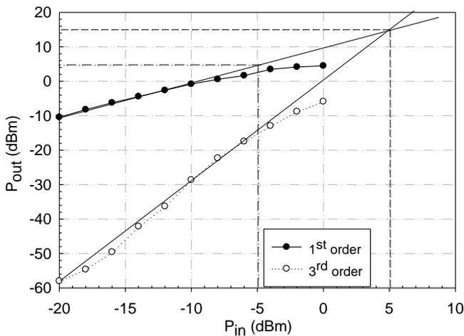
Figure 12: Measurement of IIP3
