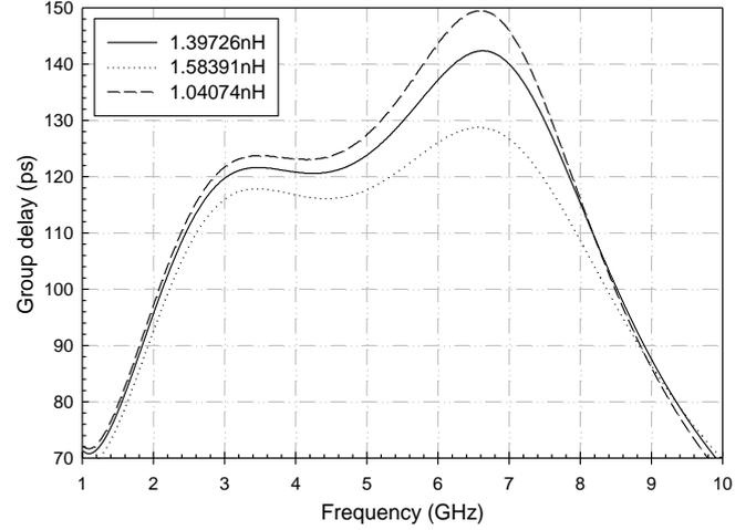
Figure 5: Effect of inductor,  $L_1$  on the group delay variation.
