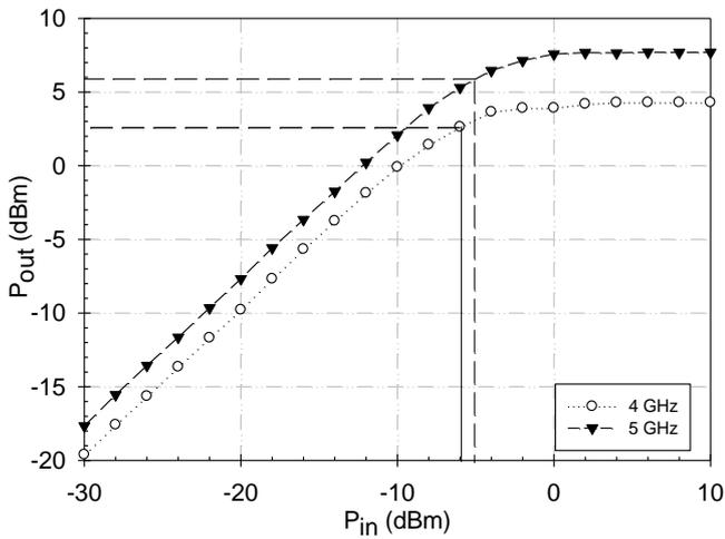
Figure 11: Measurement of P1dB
