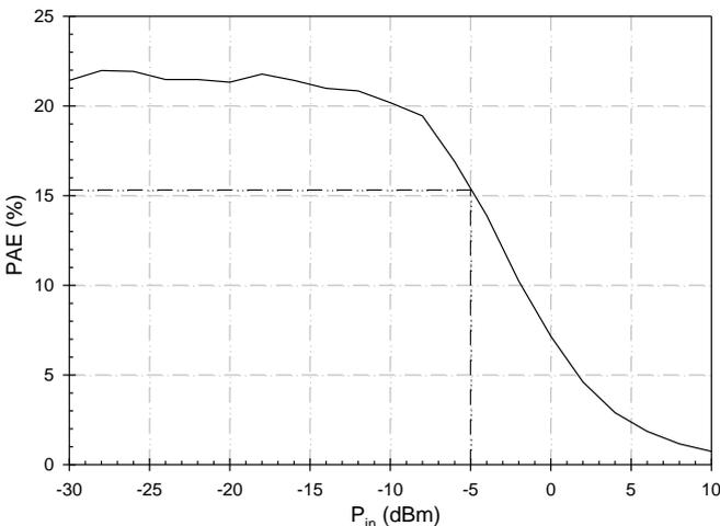
Figure 13: Measurement of PAE
