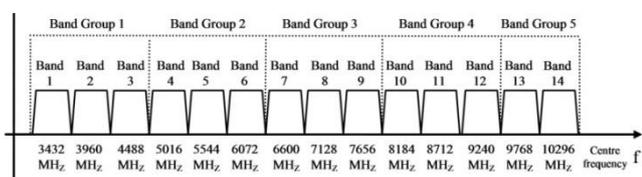
Figure 1: The band structure of MB-OFDM UWB system [4]
