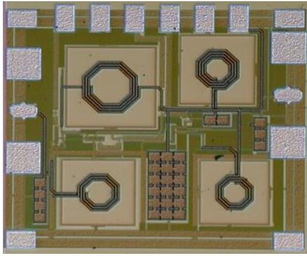
Figure 6: The proposed PA micrograph chip (0.88mm x0.78mm)
