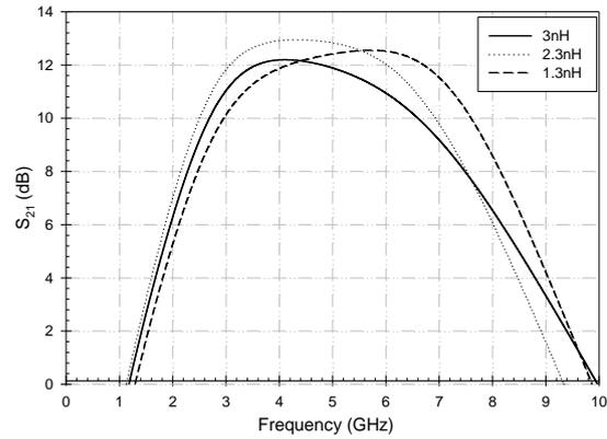
Figure 3: Effect of  $L_3$  on gain (post layout simulation)
