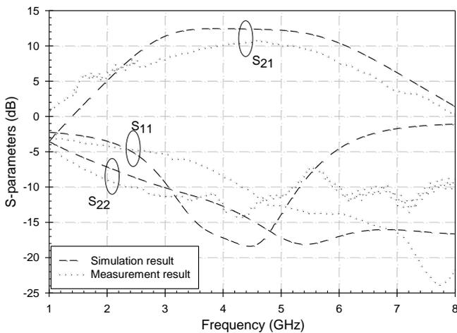
Figure 7: Measurement and simulation of S-parameters
