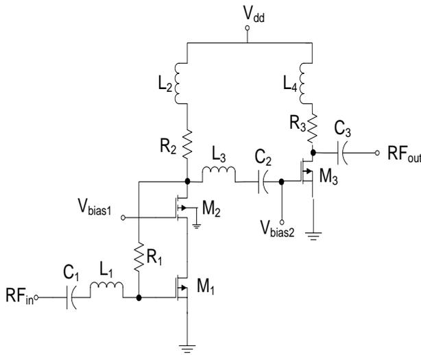
Figure 2: Proposed PA design schematic.
