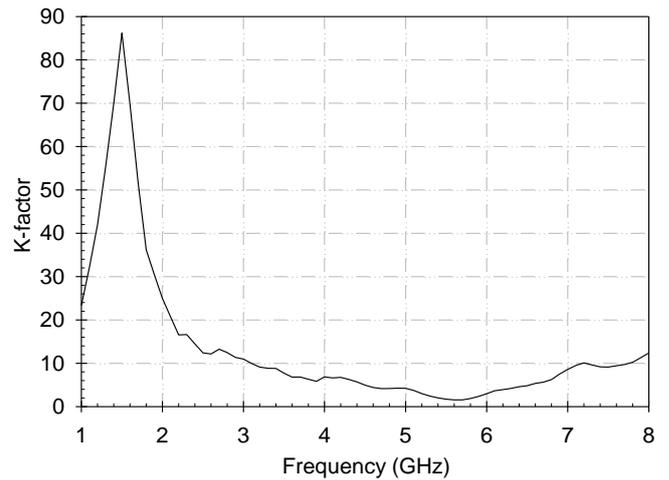
Figure 9: Measurement of stability factor (K-factor)
