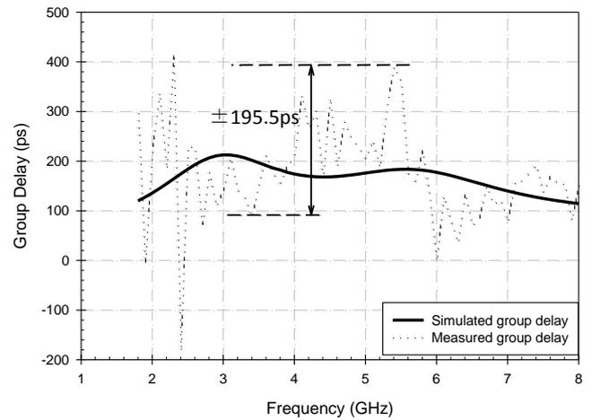
Figure 10: Measurement and simulation of group delay versus frequency
