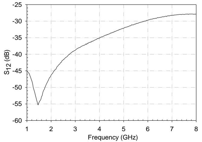
Figure 8: Measurement of reverse isolation ( $S_{12}$ )
