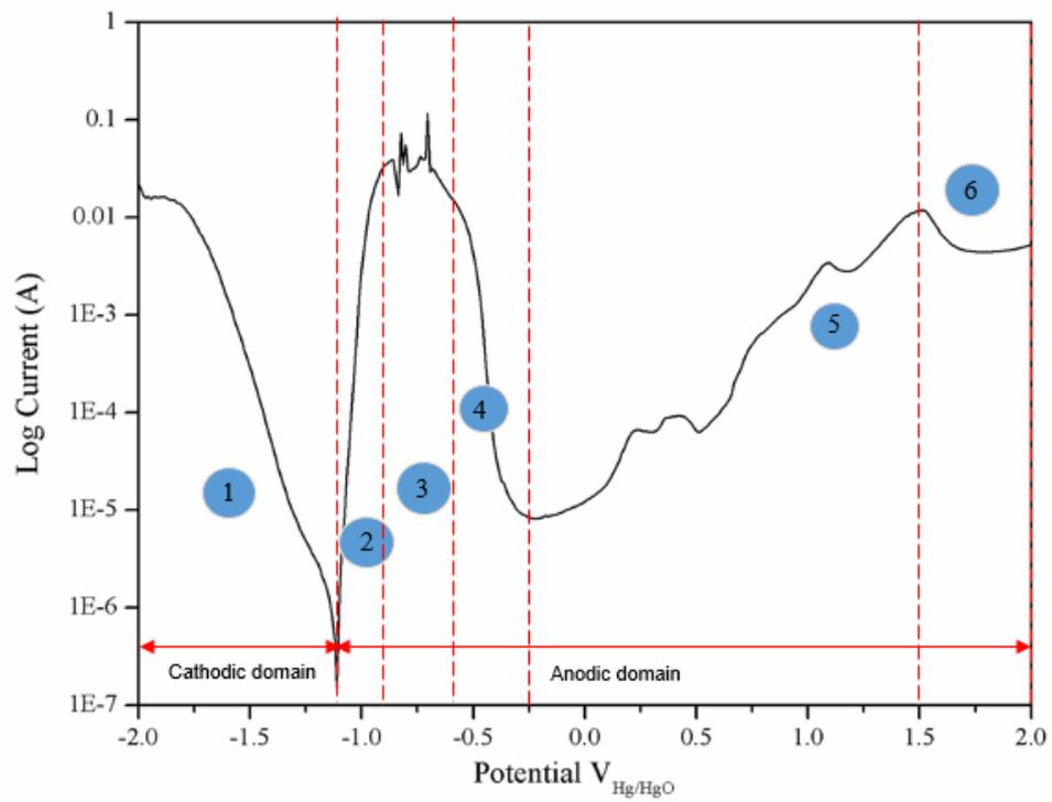
**Figure 1:** Potentiodynamic polarization of SAC305 solder in 6 M KOH solution at scan rate 1.0 mV/s
