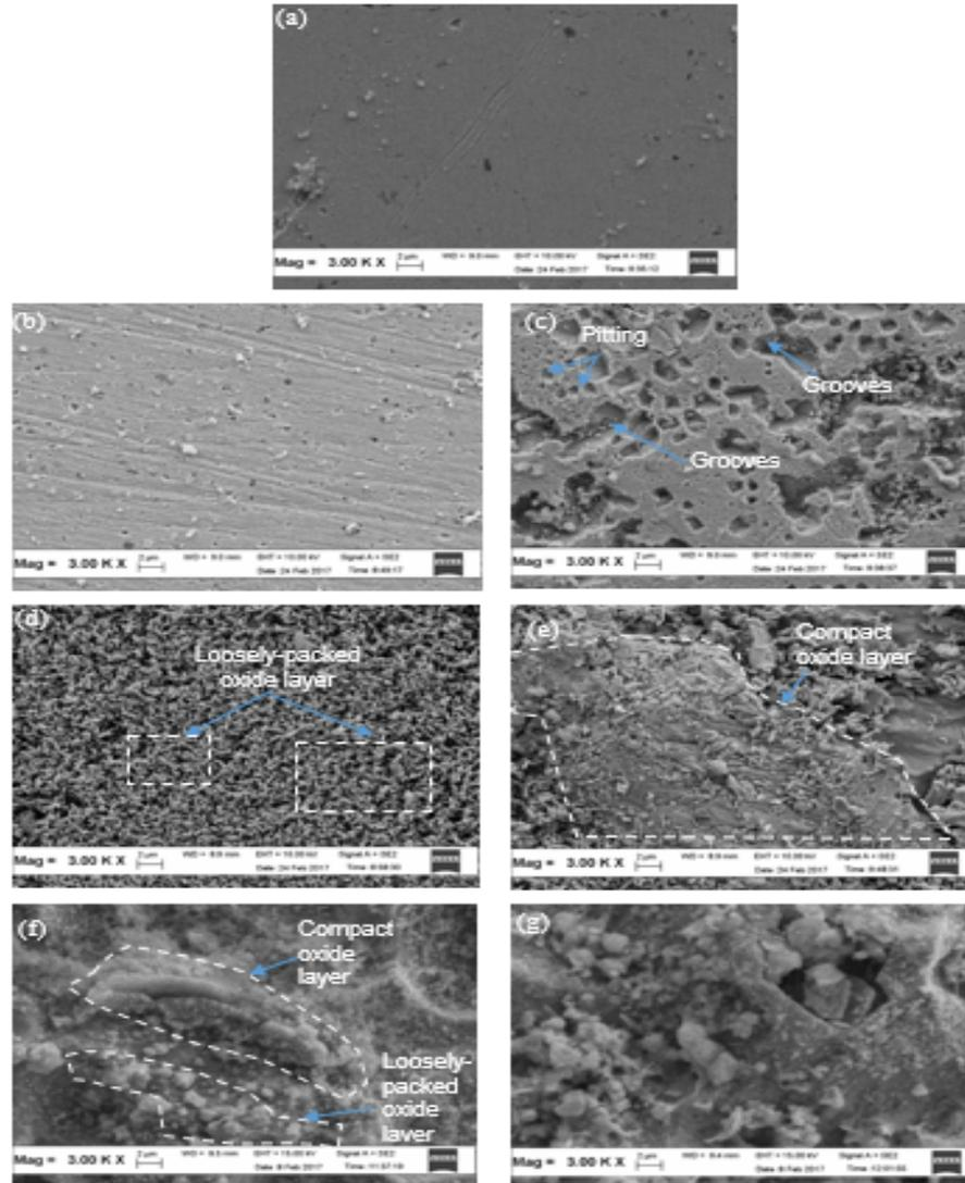
**Figure 3:** FESEM images for solder SAC305 in 6 M KOH by part: (a) as-prepared, (b) part 1, (c) part 2, (d) part 3, (e) part 4, (f) part 5 and (g) part 6
