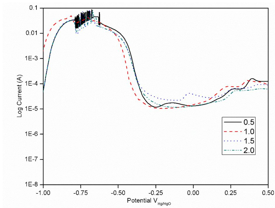
**Figure 2:** Potentiodynamic polarization curves of SAC305 solder at different scanning rate
