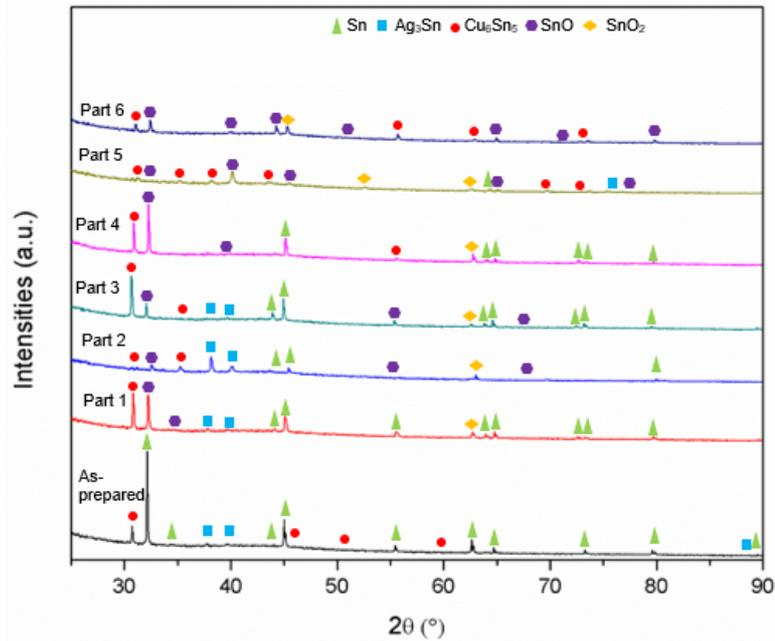
**Figure 4:** XRD pattern for solder SAC305 in 6 M KOH solution at scan rate 1.0 mV/s
