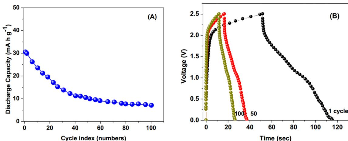
**Figure 6:** (A) Cyclic performance of the hybrid BatCap and (B) charge-discharge profile in 1, 50 100<sup>th</sup> cycles.
