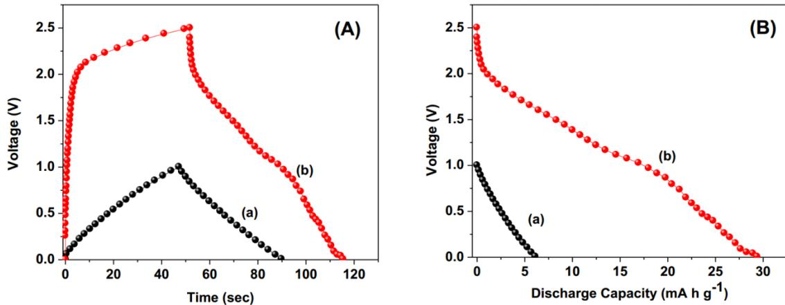
**Figure 5:** (A) Galvanostatic charge-discharge curves at  $1 \text{ mA cm}^{-2}$  ( $1 \text{ A g}^{-1}$ ), (B) Expanded representations of discharge profiles (i.e. specific capacity versus voltage profiles) of the (a) symmetric pseudocapacitor cell 1 and (b) hybrid BatCap cell 2.
