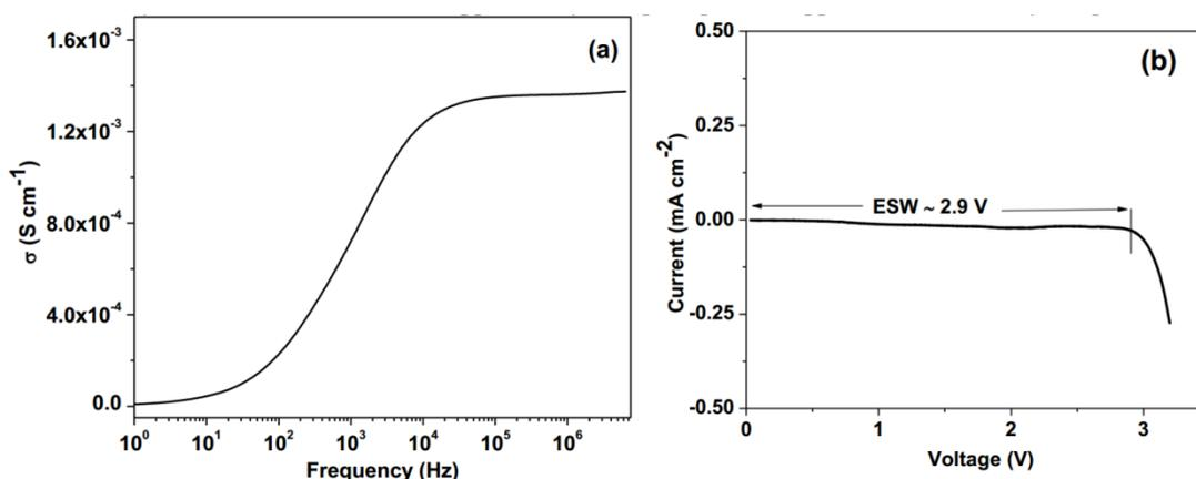
**Figure 1:** (a) Bode plot and (b) LSV response of GPE film at room temperature (27 °C).
