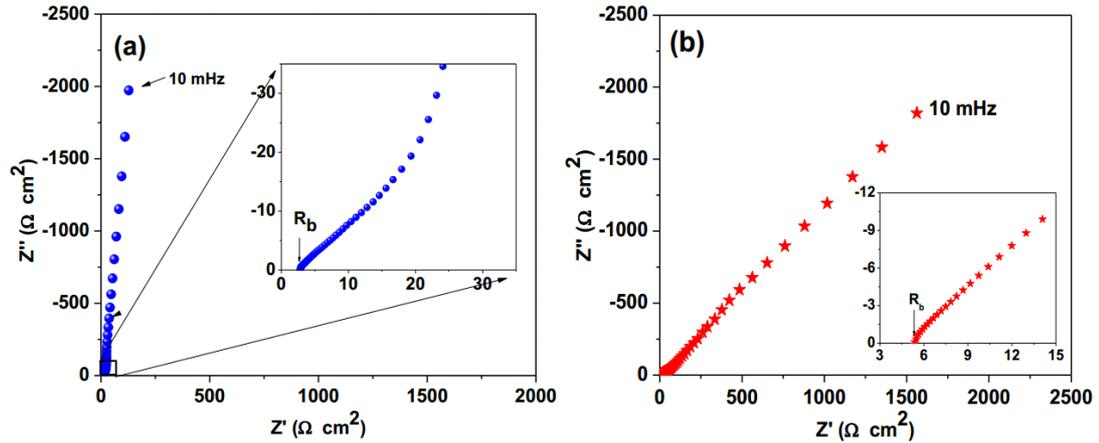
**Figure 3:** Electrochemical impedance spectra of (a) pseudocapacitor cell and (b) hybrid BatCap cell.
