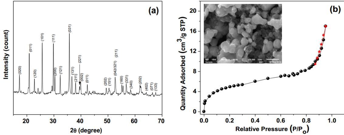
**Figure 2:** (a) XRD pattern and (b)  $N_2$ -adsorption-desorption isotherms of the pristine  $LiFePO_4$ . SEM image is shown as inset.
