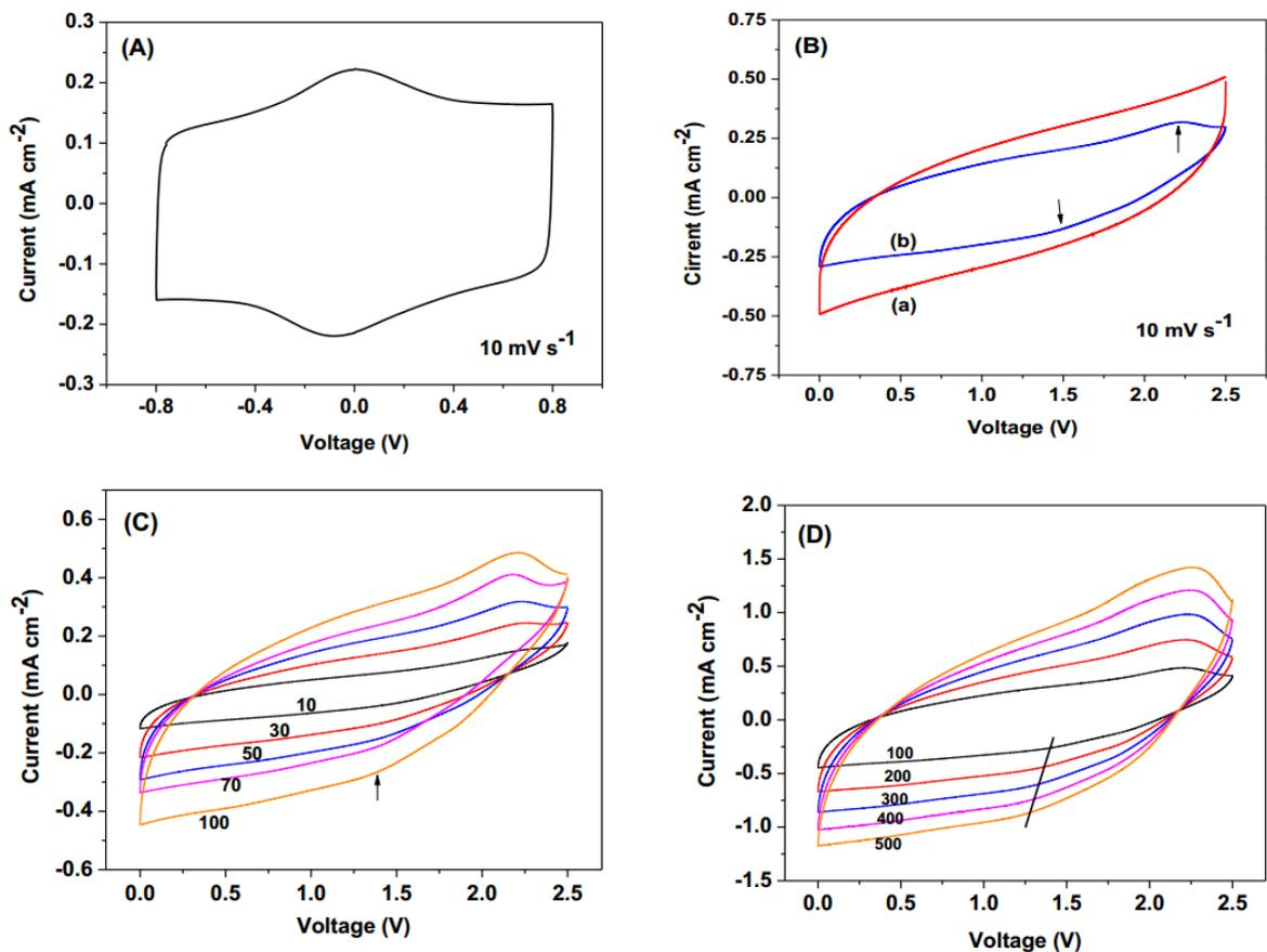
**Figure 4:** (A) Cyclic voltammogram of the pseudocapacitor cell 1, (B) Comparative CV curves of (a) cell 1 and (b) cell 2 at scan rate 10  $\text{mV s}^{-1}$ , and (C and D) CVs of hybrid BatCap cell 2 at different scan rates. Scan rates (in  $\text{mV s}^{-1}$ ) are marked on each voltammogram.
