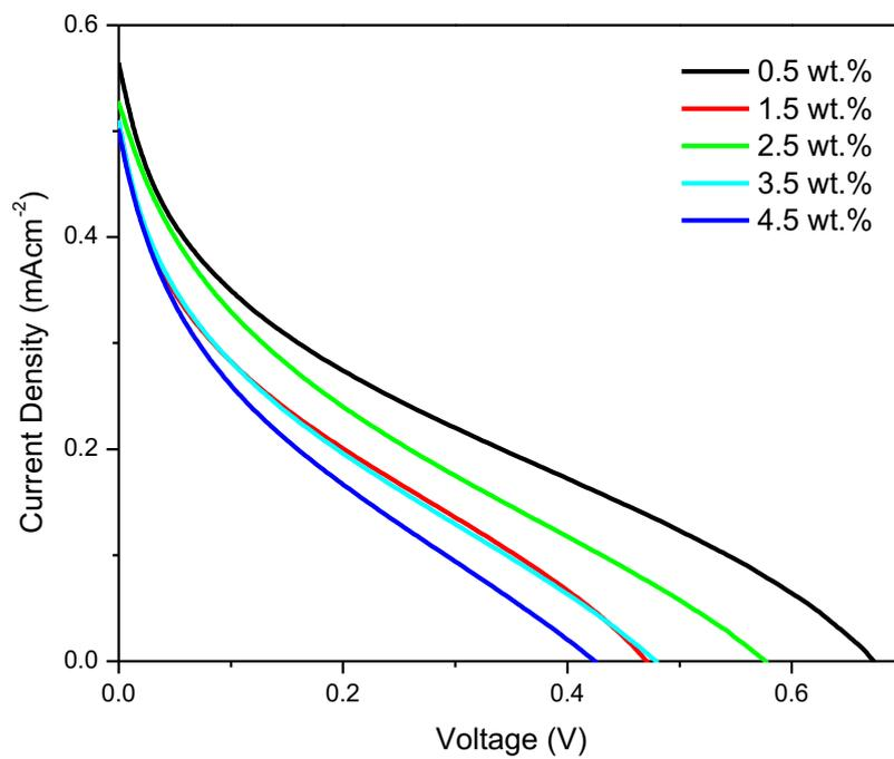
Figure 4:  $J-V$  curves under the illumination of  $100 \text{ mWcm}^{-2}$  light for the DSSCs with difference wt.% GO
