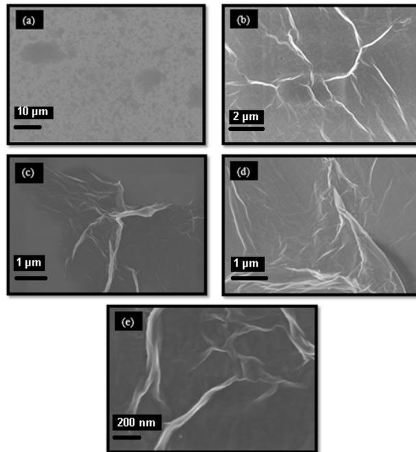
**Figure 1:** FESEM images of rGO films with various wt.% GO: (a) 0.5 wt.%, (b) 1.5 wt.% (c), 2.5 wt.%, (d) 3.5 wt.% and (e) 4.5 wt.% (10000× magnification)
