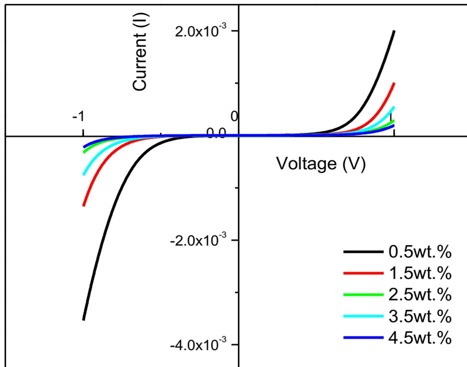
**Figure 2:**  $I$ - $V$  curves in dark for the DSSCs with various wt.% GO
