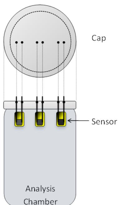
**Figure 3:** Measurement chamber, showing (for clarity) 3 of the 6 sensors
