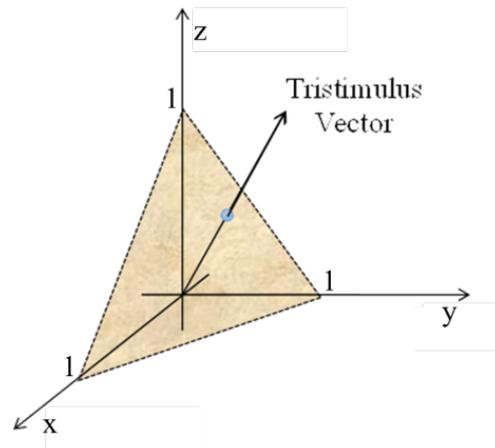
**Figure 4:** Graphical representation of the tristimulus vector and the interception point in the unitary plane
