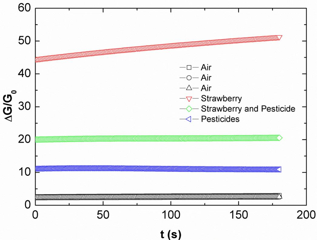
**Figure 5:** Response variation of a MWCNT based sensor when exposed to air, to a strawberry, to a pesticide treated strawberry and to only pesticide. The data for the three air samples all give a similar low value
