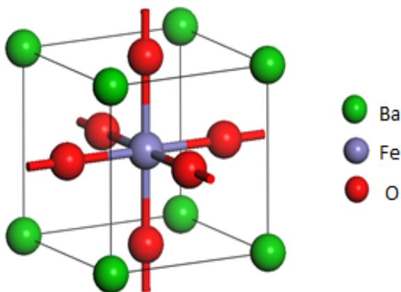
Figure 2: Crystal structure of BaFeO<sub>3</sub> unit cell
