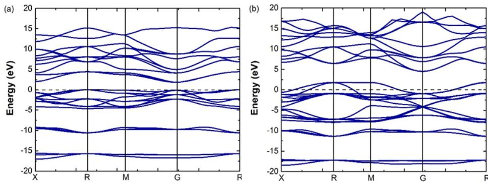
Figure 3: Band structures of (a) BaTiO<sub>3</sub> and (b) BaFeO<sub>3</sub> from LDA+U calculation
