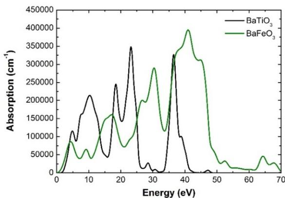
Figure 5: Absorption of BaTiO<sub>3</sub> and BaFeO<sub>3</sub> within range of photon energy
