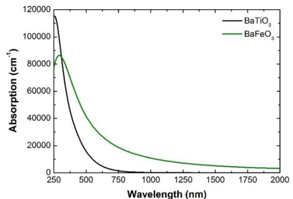
Figure 6: Absorption of BaTiO<sub>3</sub> and BaFeO<sub>3</sub> within range of wavelength
