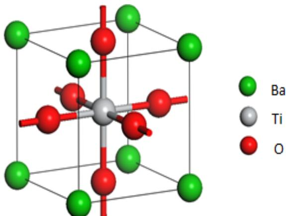
Figure 1: Crystal structure of BaTiO<sub>3</sub> unit cell
