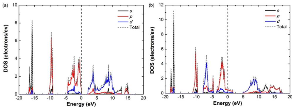
Figure 4: Density of states of a) BaTiO<sub>3</sub> and (b) BaFeO<sub>3</sub> from LDA+U calculation
