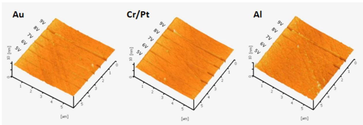
**Figure 1:** Silicon nanowires patterns using different types of tip (Au, Cr/Pt and Al) with different applied voltages (5, 6, 7V, 8, and 9 V) at 0.3 μm/s writing speed
