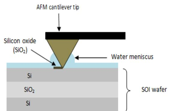
**Figure 3:** Concept of LAO process on silicon-on-insulator wafer
