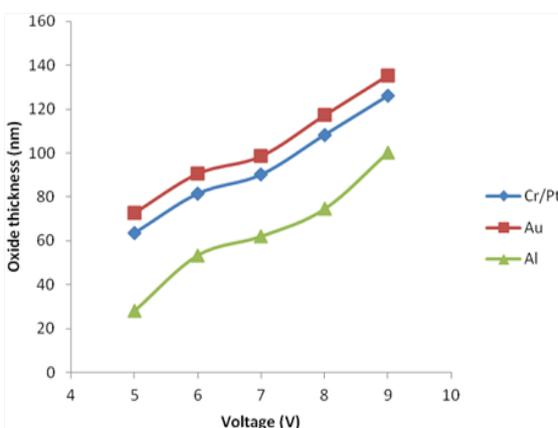
**Figure 2:** Relation of oxide thickness with different applied voltages for different types of AFM cantilever tips
