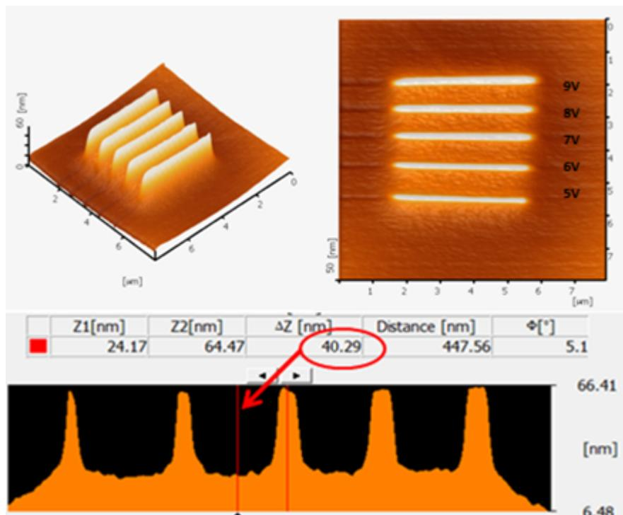
**Figure 5:** AFM profile image of silicon nanowires pattern using Au coated tip after etching process
