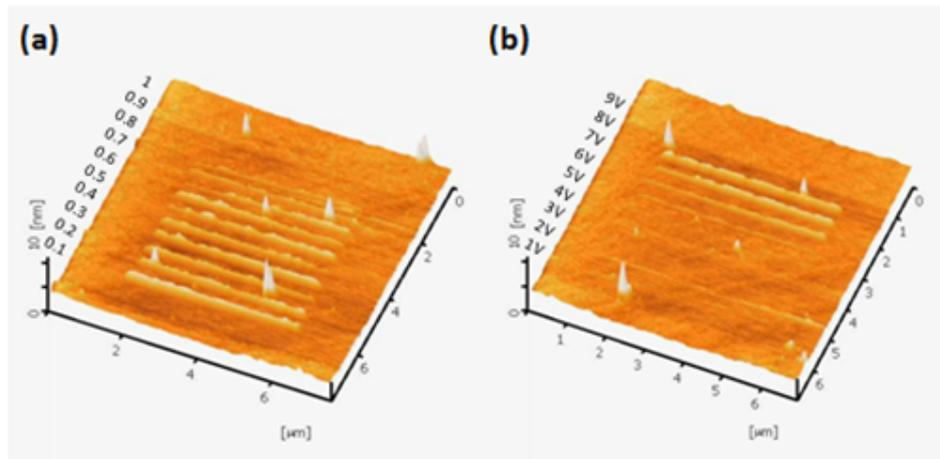
**Figure 4:** Silicon nanowires patterns at (a) different writing speed (1.0  $\mu\text{m/s}$ , 0.9  $\mu\text{m/s}$ , 0.8  $\mu\text{m/s}$ , 0.7  $\mu\text{m/s}$ , 0.6  $\mu\text{m/s}$ , 0.5  $\mu\text{m/s}$ , 0.4  $\mu\text{m/s}$ , 0.3  $\mu\text{m/s}$ , 0.2  $\mu\text{m/s}$ , and 0.1  $\mu\text{m/s}$ ) (b) different applied voltages (9, 8, 7, 6, 5, 4, 3, 2, and 1 V) using Au tip
