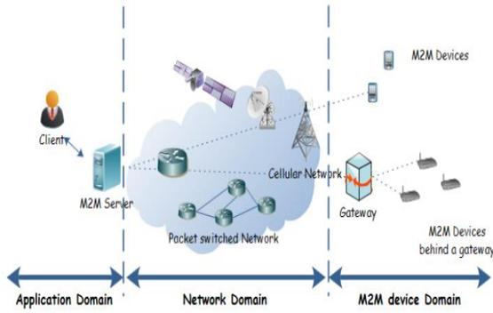
Figure 2: General Architecture of an M2M Application [4]
