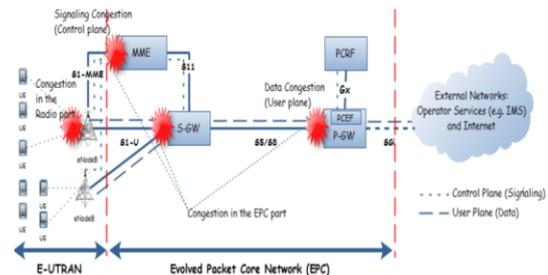
Figure 1: Blocking in the LTE-A Network [3]
