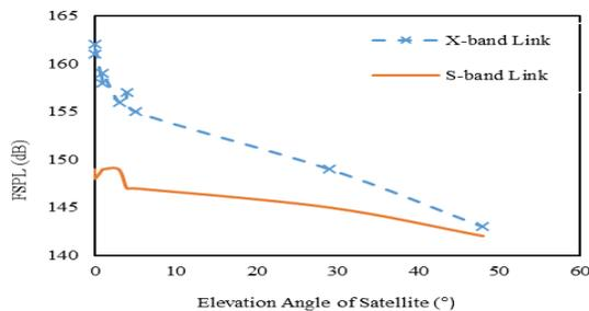
Figure 4: FSPL Estimation values for S-band and X-band link
