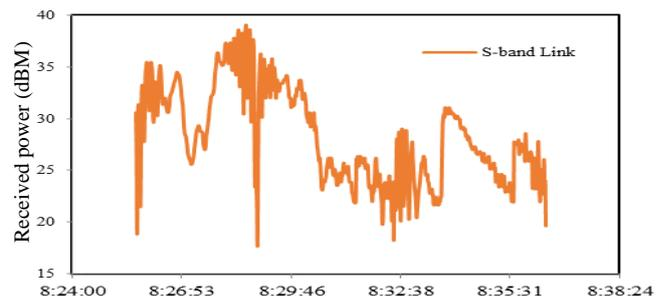
Figure 2: RazakSAT Received Power for S-band Link
