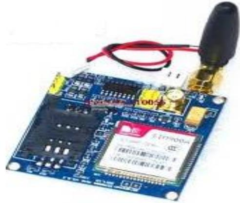
Figure 4: Simcom GSM SIM900A [21]
