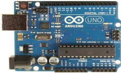
Figure 2: Arduino UNO board [20]
