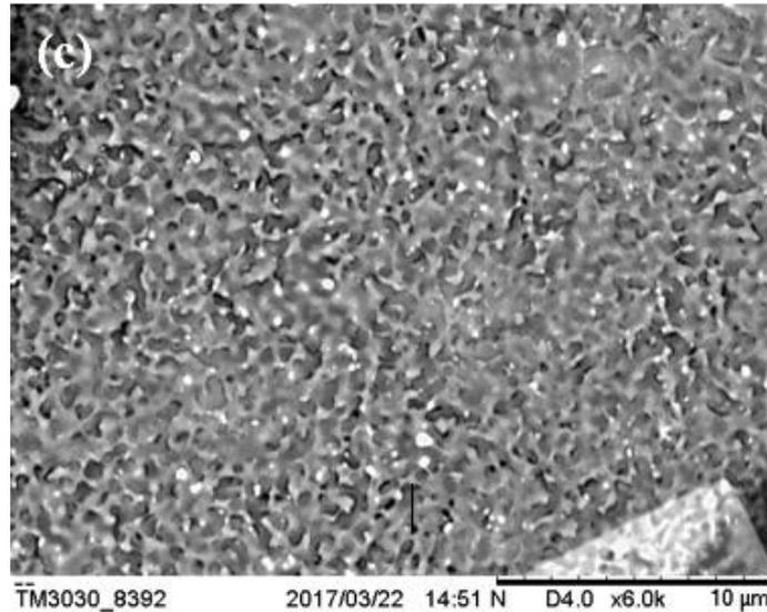
Figure 2: Different concentration shows different interspacing between the particles; SEM characterization for TiO<sub>2</sub> (a) 0.15M, (b) 0.20M, (c) 0.25M
