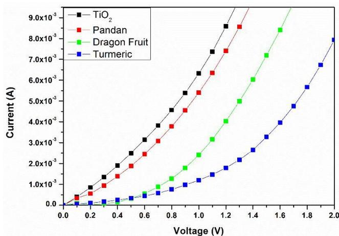
Figure 3: I-V Characteristics for 0.25 M of TiO<sub>2</sub> with different dyes
