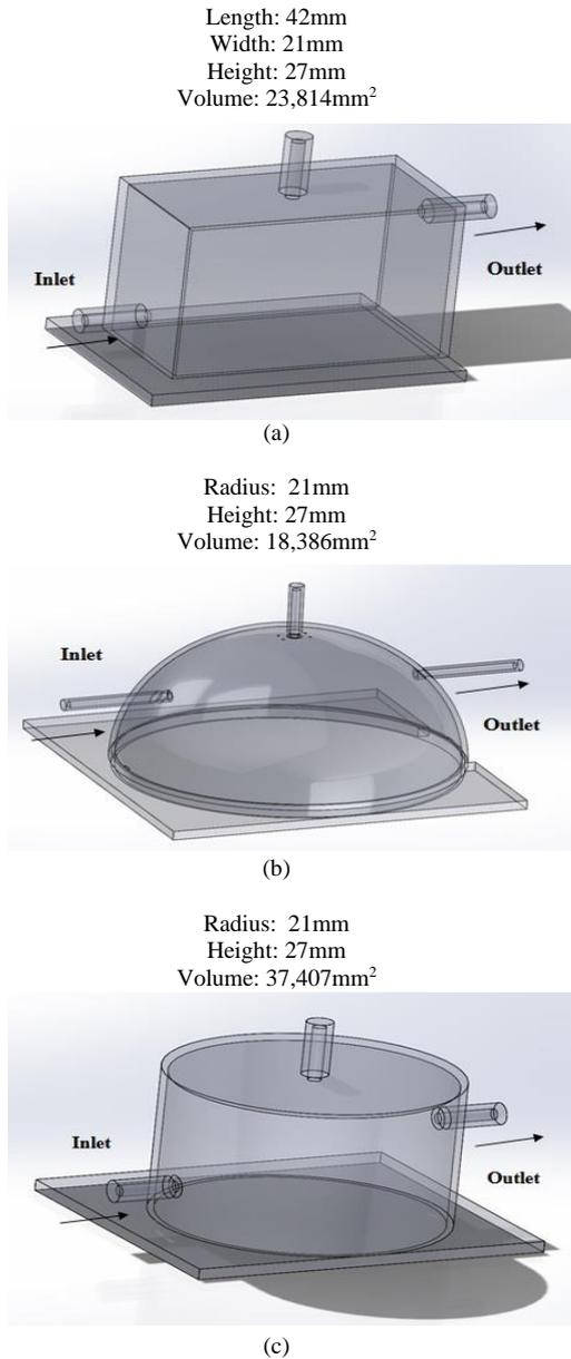
Figure 1: Shapes, measurements and volumes of the (a) rectangular, (b) hemisphere and (c) cylindrical sensing chambers
