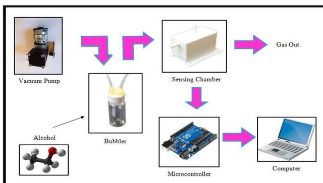
Figure 2: Detection stage of an E-Nose system which consists of a bubbler, sensing chamber and gas sensor (in the sensing chamber)
