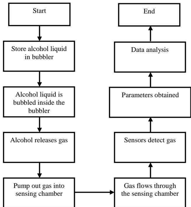
Figure 3: Sensing process of the detection stage in an E-Nose system
