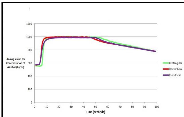
Figure 6: Sensor's response time (alcohol concentration versus time) for different sensing chambers (rectangular, hemisphere and cylindrical)
