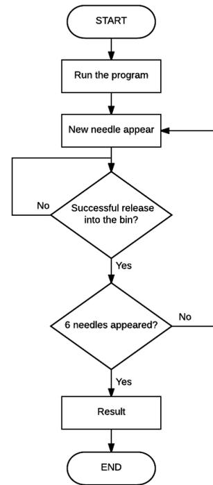
Figure 2: Needle grasping module flowchart
