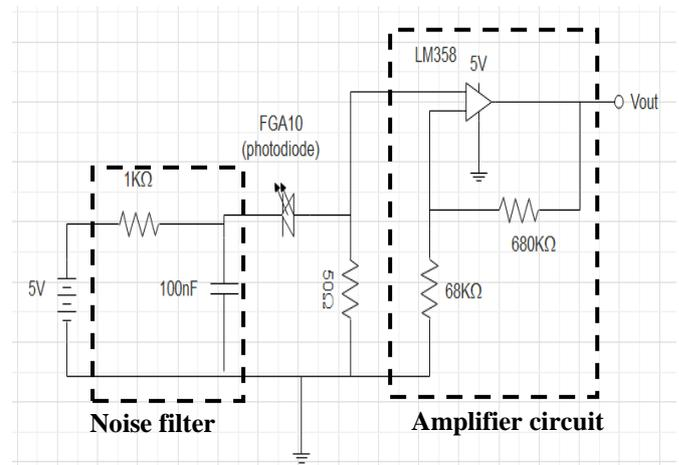
Figure 2: Filter and amplifier circuit
