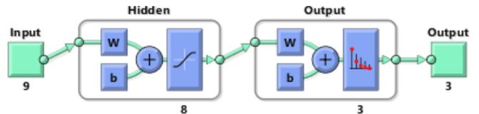
Figure 7: Architecture of neural network
