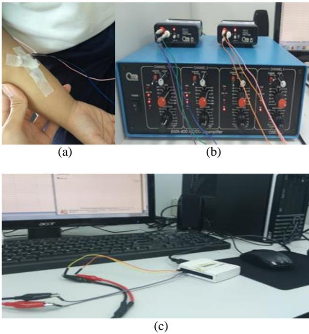
Figure 2: (a) Electrode placement on the subject (b) BMA-400 Bio-amplifier and ISO-Z amplifier (c) National Instrument USB-6009 connected to computer and the input from bio-amplifier
