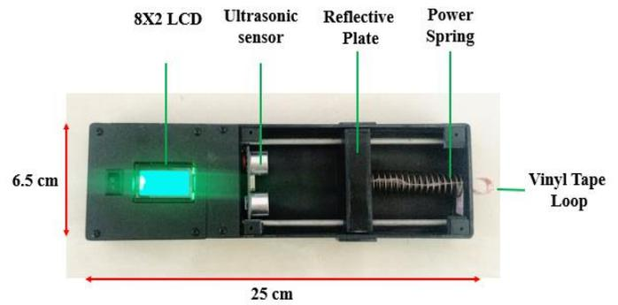
Figure 3: Overall structure of the developed device
