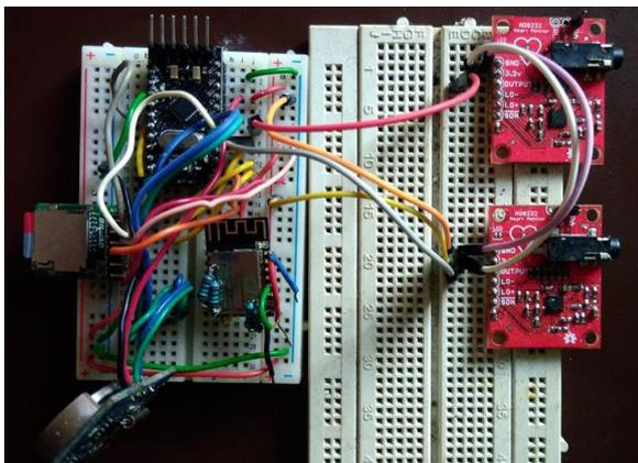
Figure 6: Wireless ECG device prototype
