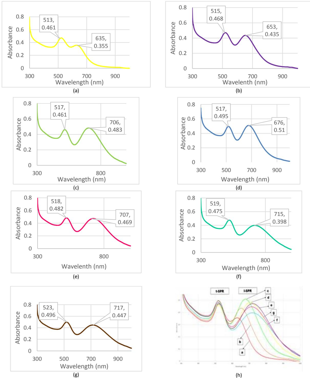
Figure 7: The UV-Vis absorption spectra by using different molarity of  $\text{AgNO}_3$ . (a) 0.5 mM  $\text{AgNO}_3$  (b) 1.0 mM  $\text{AgNO}_3$  (c) 2.0 mM  $\text{AgNO}_3$  (d) 3.0 mM  $\text{AgNO}_3$  (e) 4.0 mM  $\text{AgNO}_3$  (f) 5.0 mM  $\text{AgNO}_3$  (g) 6.0 mM  $\text{AgNO}_3$  (h) All concentration of  $\text{AgNO}_3$
