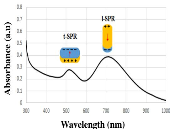
Figure 6: An example of AuNRs surface plasmon resonance with schematic describing the electron oscillations along the two axes within the nanorods [10].
