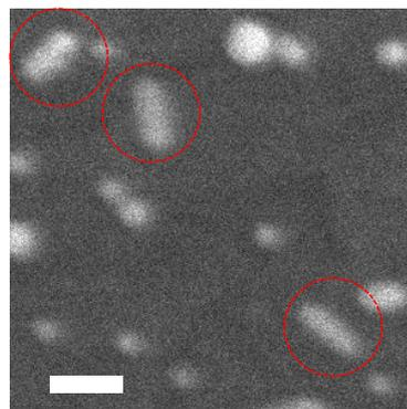
Figure 5: The formation of AuNRs on ITO substrate. Scale: 100 nm
