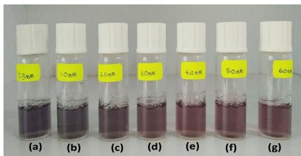
Figure 4: The different colors for different concentrations of  $\text{AgNO}_3$  added into the growth solution. (a) 0.5 mM  $\text{AgNO}_3$  (b) 1.0 mM  $\text{AgNO}_3$  (c) 2.0 mM  $\text{AgNO}_3$  (d) 3.0 mM  $\text{AgNO}_3$  (e) 4.0 mM  $\text{AgNO}_3$  (f) 5.0 mM  $\text{AgNO}_3$  (g) 6.0 mM  $\text{AgNO}_3$
