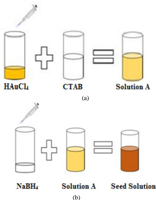
Figure 1: Preparation of Seeding Process for AuNRs. (a)  $\text{HAuCl}_4$  mix with CTAB, (b)  $\text{NaBH}_4$  added to the  $\text{HAuCl}_4$  mix with CTAB
