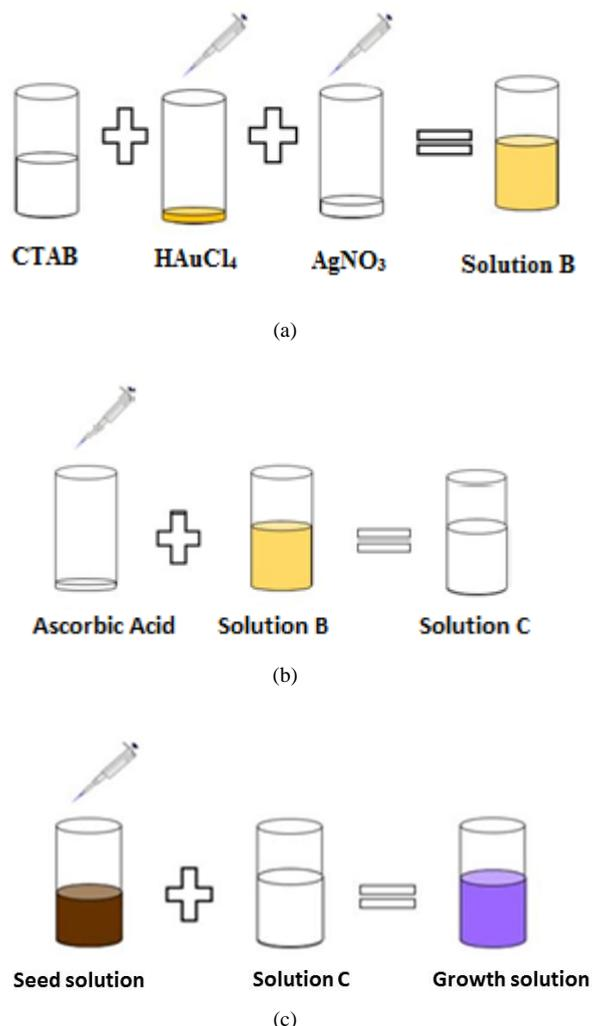
Figure 2: Preparation of growth process for AuNRs. (a) Mixture of CTAB,  $\text{HAuCl}_4$  and  $\text{AgNO}_3$  (Solution B), (b) Ascorbic acid added to the Solution B (Solution C) and (c) Seed solution added to the mixture of Solution C.
