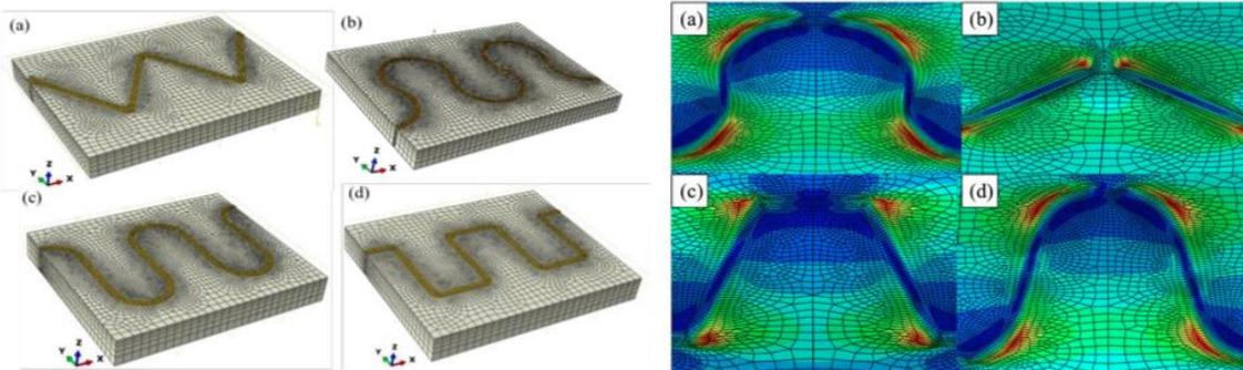
Figure 5: Left: Finite element modelling of Stretchable Electronics. (a) Zigzag shape structure (b) Horseshoe shape structure, (c) U shape structure (d) Rectangle shape structure<sup>13</sup>. Right: Von Mises stress at 60% tensile strain. (a) horseshoe shape structure (b) Zigzag shape structure (c) rectangle shape structure (d) U shape structure<sup>13</sup>
