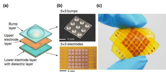
Figure 8: (a) Single capacitive sensor (b) 3x3 array of bumps and 3x3 array of electrodes (c) Flexible tactile sensors on substrate [18]
