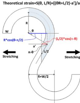
Figure 1: Concepts of a serpentine routing [9]
