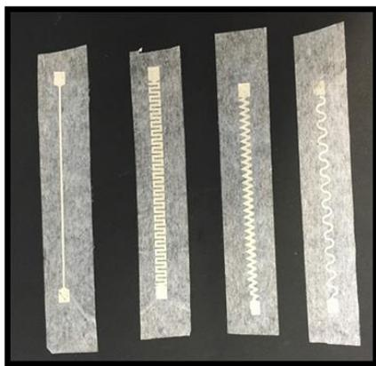
Figure 3: Screen-printed electrodes on Micropore
