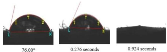
Figure 4: Contact angle measurement and time taken for Malaysian batik fabric to absorb water for 5 seconds of APPJ plasma treatment.
