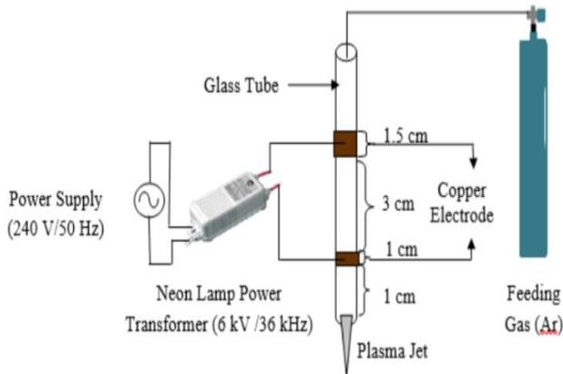
Figure 1: Configuration of atmospheric pressure plasma needle jet using copper electrodes and neon transformer power source. Argon gas flow is fixed at 50 L/min.
