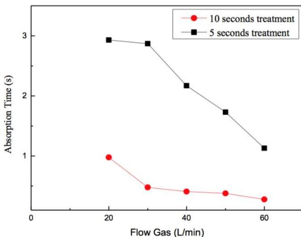
Figure 6: Water absorption time after APPJ treatment for 5 seconds and 10 seconds and various argon flow rates.
