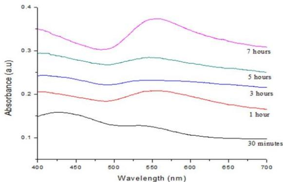
Figure 5: Optical absorption spectrum for 5 different growth time.
