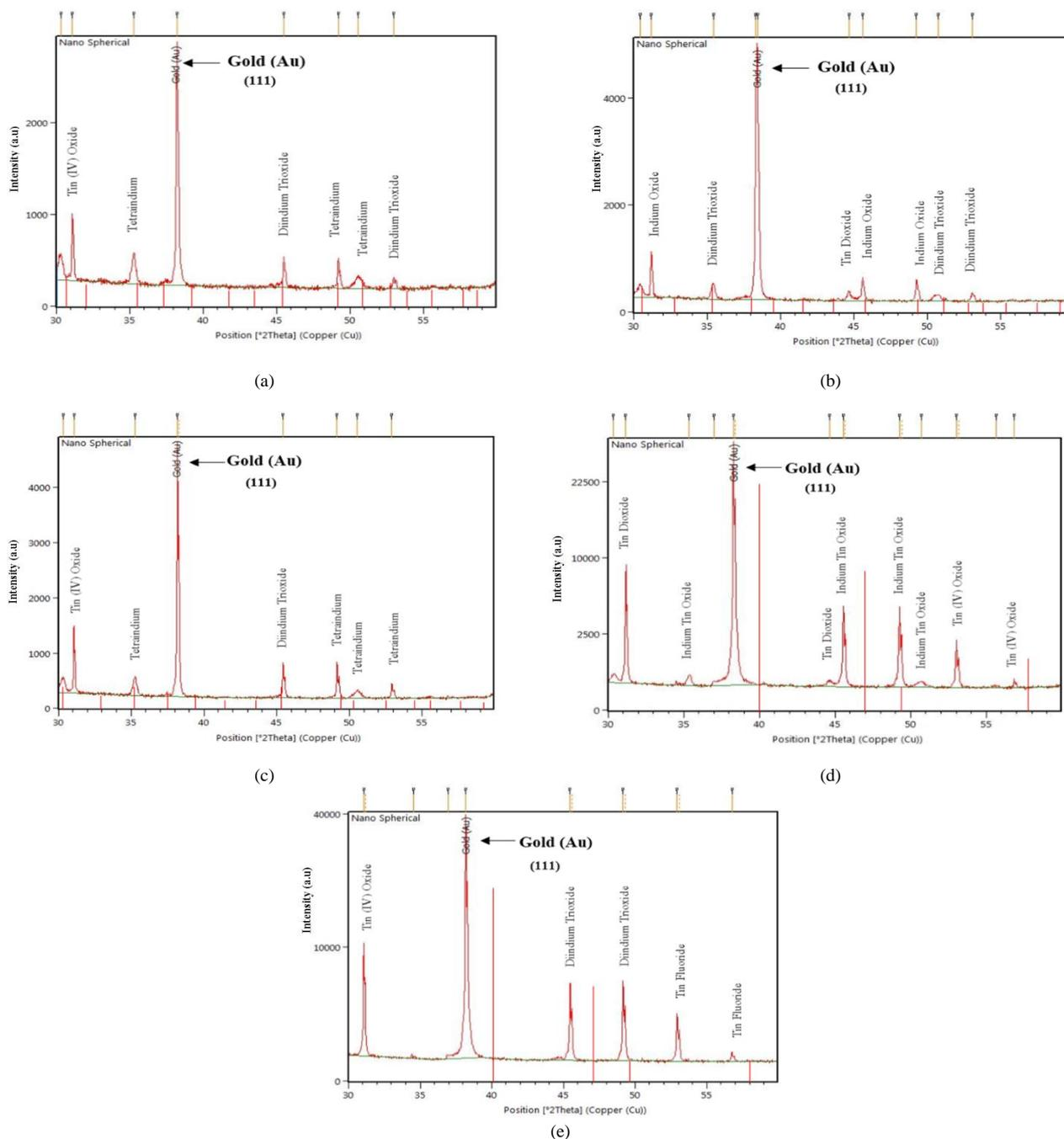
Figure 4: XRD spectra of gold nanosphericals deposited on (a) 30 minutes, (b) 1 hour, (c) 3 hours, (d) 5 hours and (e) 7 hours of growth time.
