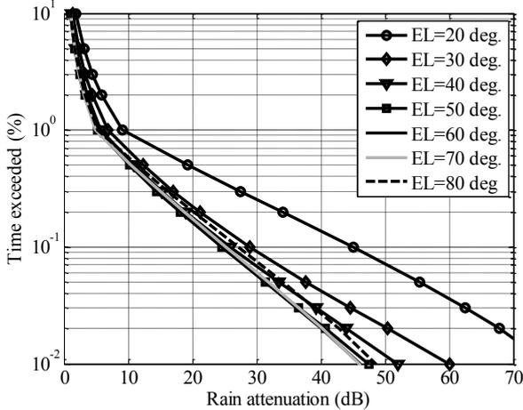
Figure 6: CCDF of rain attenuation predicted by ITU-R P.618-12 model at 20.245 GHz.
