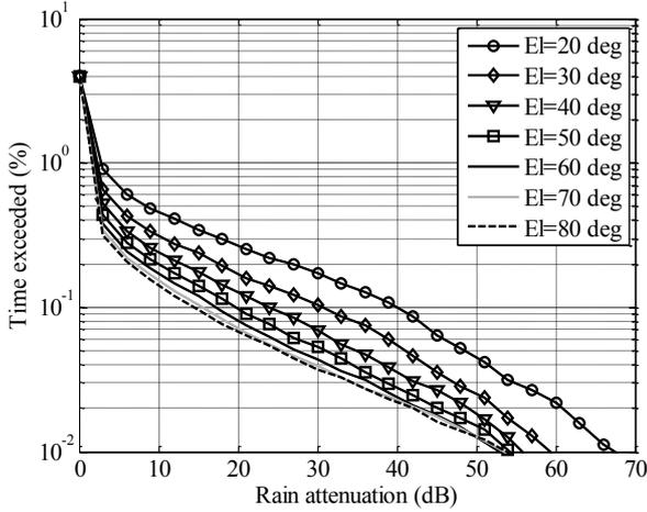
Figure 5: CCDF of rain attenuation predicted by SST model at 20.245 GHz.
