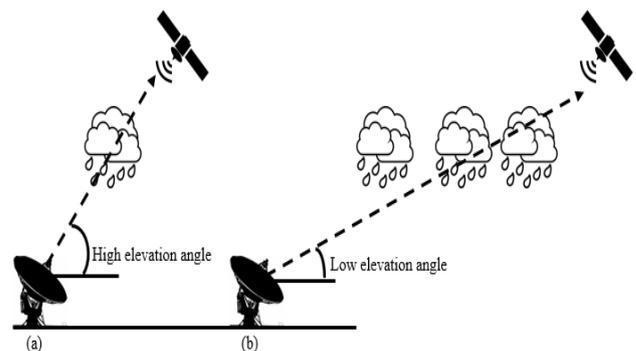
Figure 1: Different path length geometries as a function of link elevation angles. (a) High elevation angle (b) Low elevation angle [3]
