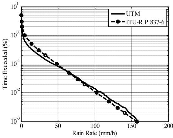
Figure 2: CCDF comparison of rainfall rate between data collected at UTM and predicted by ITU-R P.837-6 model.
