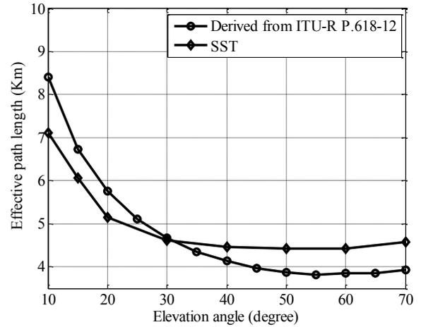
Figure 7: Effective path length as a function of elevation angle. Comparison between SST and ITU-R model.
