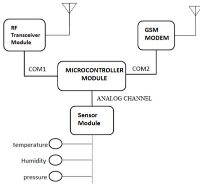
Figure 6: Acquisition Node with GSM Modem Block Diagram
