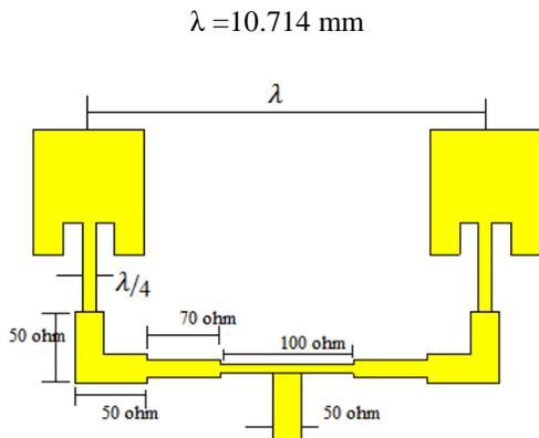
Figure 2: The front view of 2x1 patch antenna
