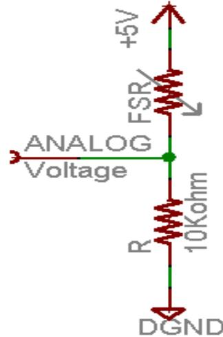
Figure 6: Circuit for FSR implementation
