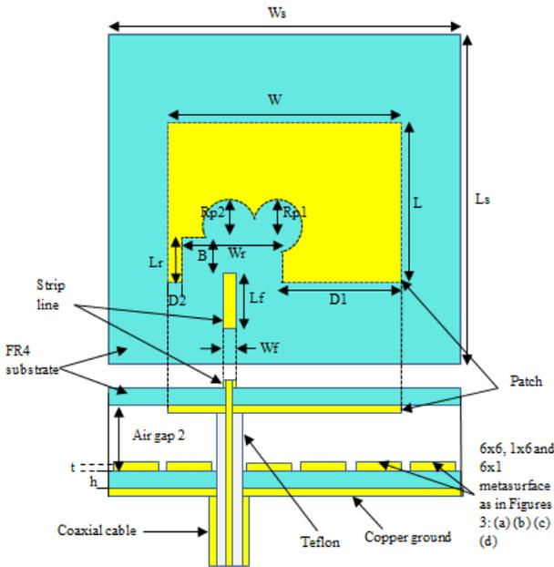
Figure 2: Configuration of L-probe right-handed circular polarized (RHCP) rectangular MSA with dual notch and metasurface in vertical view
