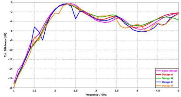
Figure 7: Comparison of simulated total efficiency for RHCP antenna without and with different MS design – simulation
