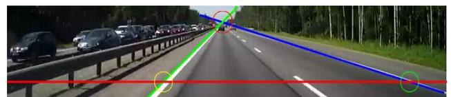
Figure 7: Point of intersection with reference line.
