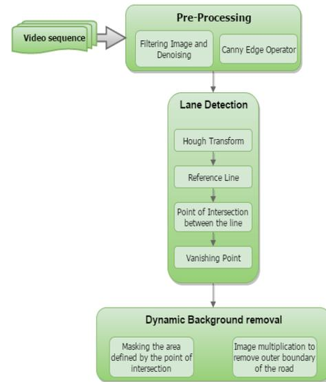
Figure 1: The overall flow of the system
