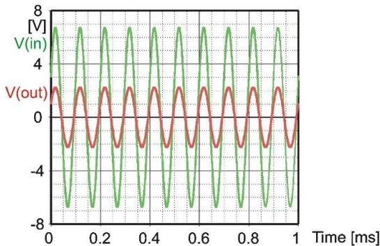
Figure 3: Transient analysis of Wien Bridge Oscillator
