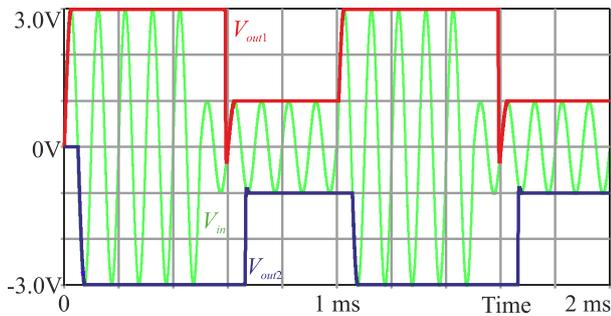
Figure 8: Transient analysis of the modified envelope detector.
