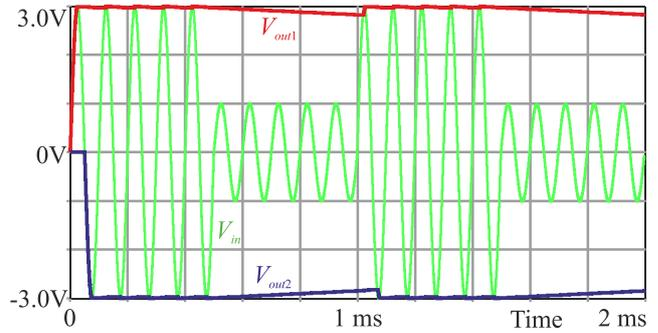
Figure 6: Transient analysis of the envelope detector with lower  $R_{off} = 100 \text{ k}\Omega$ .
