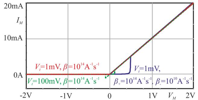
Figure 3: Current-voltage characteristic of the BMST element with various threshold voltages and slopes.
