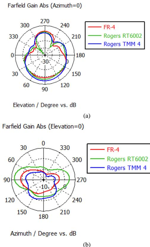
Figure 11: Simulated radiation pattern of dual band printed dipole antennas at 5 GHz. (a) Elevation and (b) azimuthal plane
