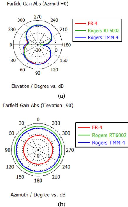
Figure 10: Simulated radiation pattern of dual band printed dipole antennas at 2.4 GHz (a) Elevation and (b) azimuthal plane
