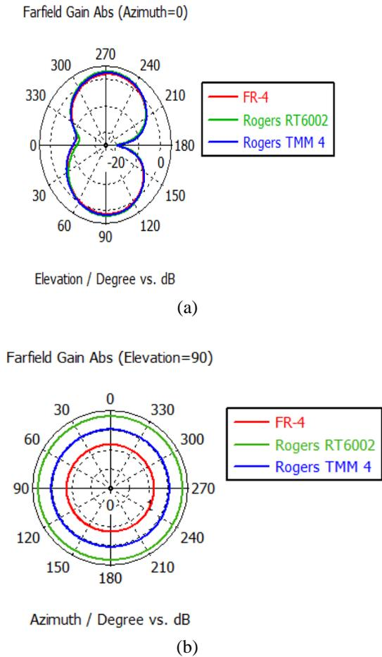
Figure 6 Simulation radiation pattern of single band printed dipole antennas. (a) Elevation plane (b) Azimuthal plane
