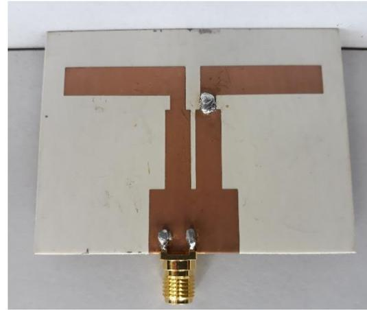
Figure 7: Fabricated of single band printed dipole antenna at 2.4GHz on Rogers RT6002 substrate.
