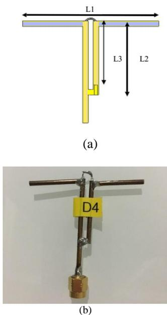
Figure 2: (a) Simulated antenna using CST (b) Fabricated dipole antenna with balun at 2.4 GHz.
