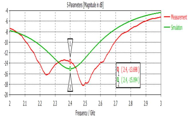
Figure 8: S11 simulation and measurement results for single band printed dipole antenna on Rogers RT6002 substrate.
