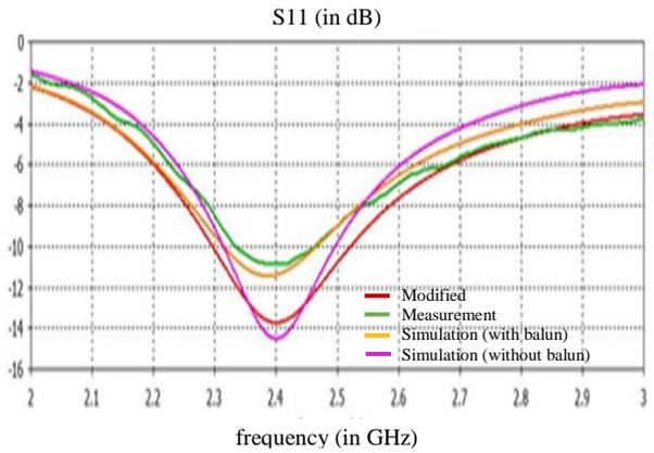
Figure 3: Return loss graph of all wire dipole
