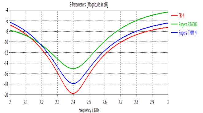
Figure 5: Return loss graph of single band printed dipole antennas.
