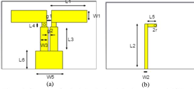
Figure 4: Geometry of a single band printed dipole antenna at 2.4GHz. (a) Top and (b) Bottom
