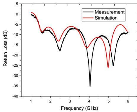
Figure 13: S11 simulation and measurement results for single band printed dipole antenna on Rogers RT6002 substrate.
