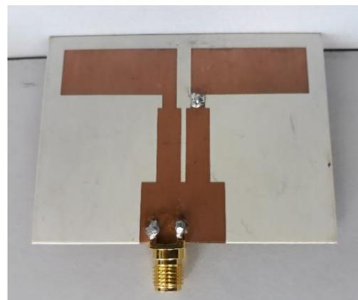
Figure 12: Fabricated of single band printed dipole antenna at 2.4GHz on Rogers RT6002 substrate
