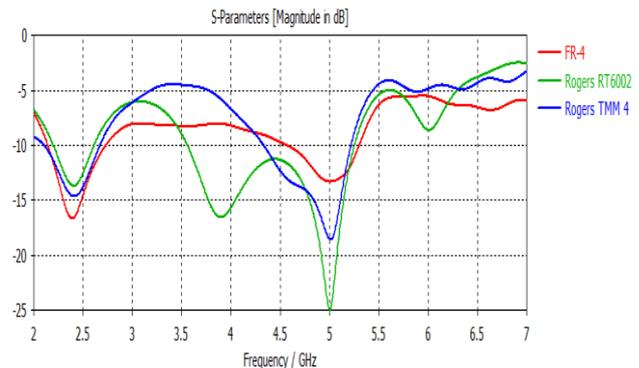
Figure 9: Return loss of dual band printed dipole antennas.
