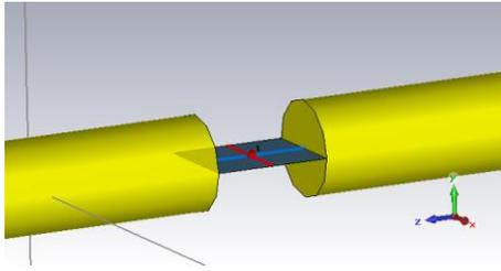
Figure 1: A simple wire dipole with discrete port
