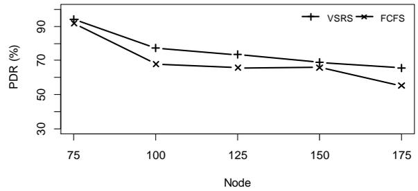
Figure 5: The average packet delivery ratio over different node densities.
