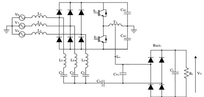
Figure 1: The three-phase AC-DC CIHRC
