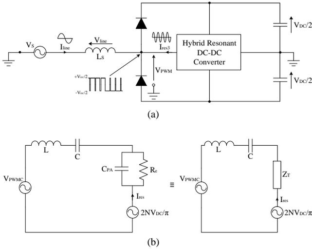
Figure 2: (a) Single leg of converter fed by hybrid resonant converter, (b) Fundamental frequency equivalent circuit for the half-bridge hybrid resonant converter
