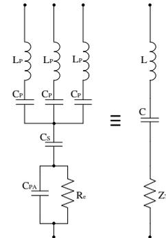
Figure 3: Equivalent resonant circuit topologies for zero-sequence harmonics
