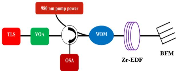
Figure 1: The configuration setup of double-pass amplification
