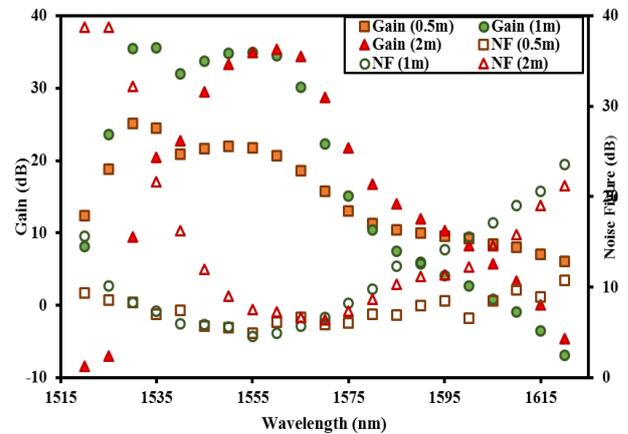
Figure 4: Gain and noise figure of the double-pass Zr-EDF by using optical circulator as the reflector for different lengths of gain medium with input signal fixed at -30 dBm
