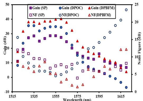
Figure 2: Gain and noise figure spectra for the single and double pass Zr-EDFA for both reflectors at the low input signal power of -30 dBm
