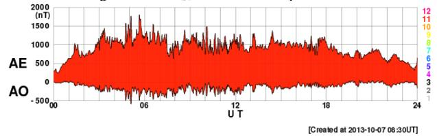
Figure 9: The  $A_E$  Index on storm period 2013.
