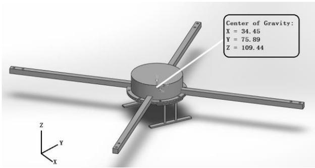
Figure 4: Center of Gravity
