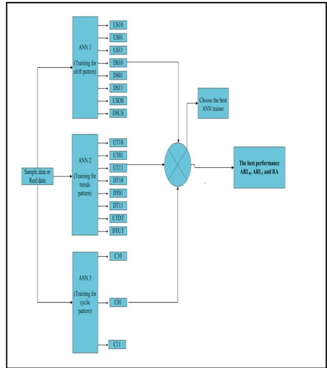
Figure 4: The CCPR scheme using modular neural network
