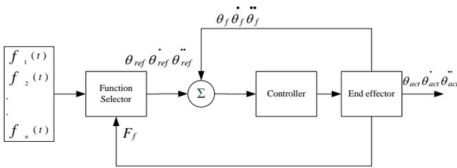
Figure 2: KUKA Youbot rehabilitation system block diagram
