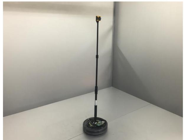
Figure 3: SP360 camera mounted on iRobot Create2
