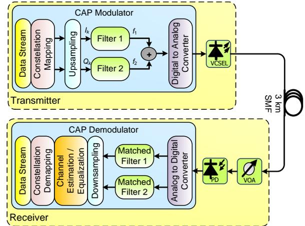
Figure 1: CAP transmission systems
