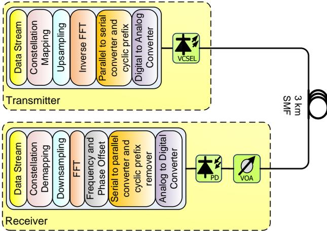
Figure 3: DMT transmission systems
