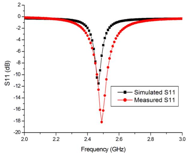
Figure 12: Simulated and measured return loss of HMA with EBG.
