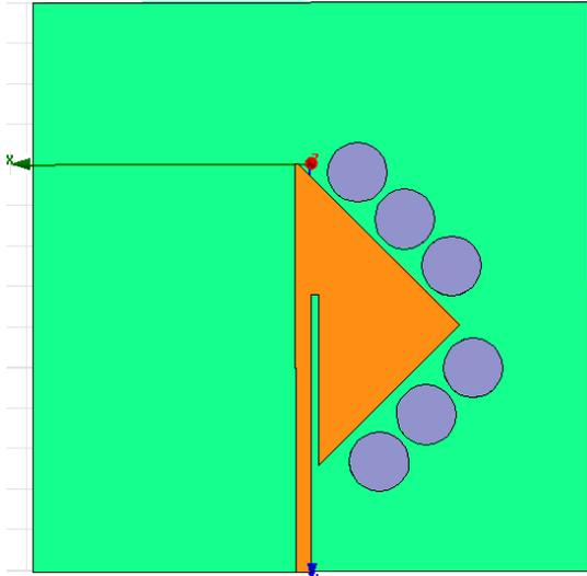
Figure 8 Simulation model of HMA with circular shape EBG
