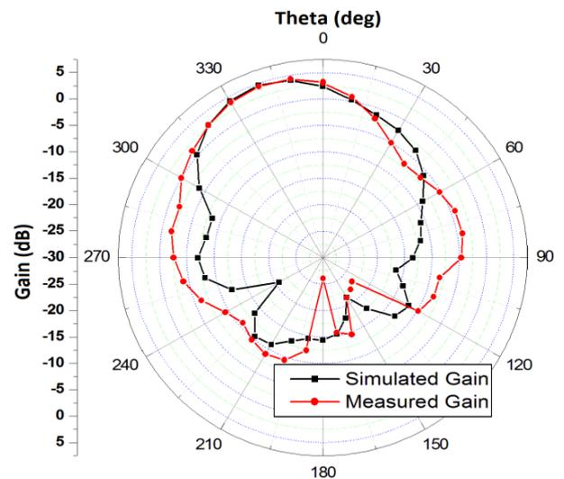
Figure 13: Simulated and measured Gain of HMA with EBG.
