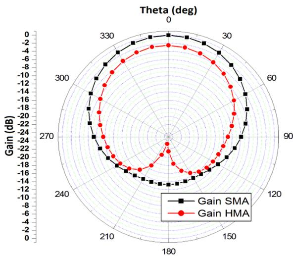
Figure 6: Simulated gain for square microstrip antenna (SMA) and Half Microstrip antenna (HMA)
