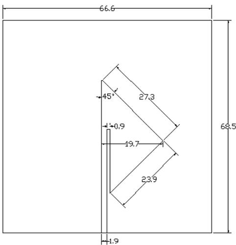
Figure 3: Geometry of half microstrip antenna (HMA) (all dimensions are in mm)
