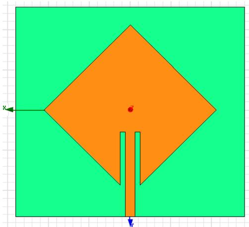
Figure 2: Simulation model of square microstrip antenna (SMA)
