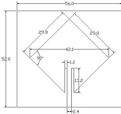
Figure 1: Geometry of square microstrip antenna (all dimensions are in mm)
