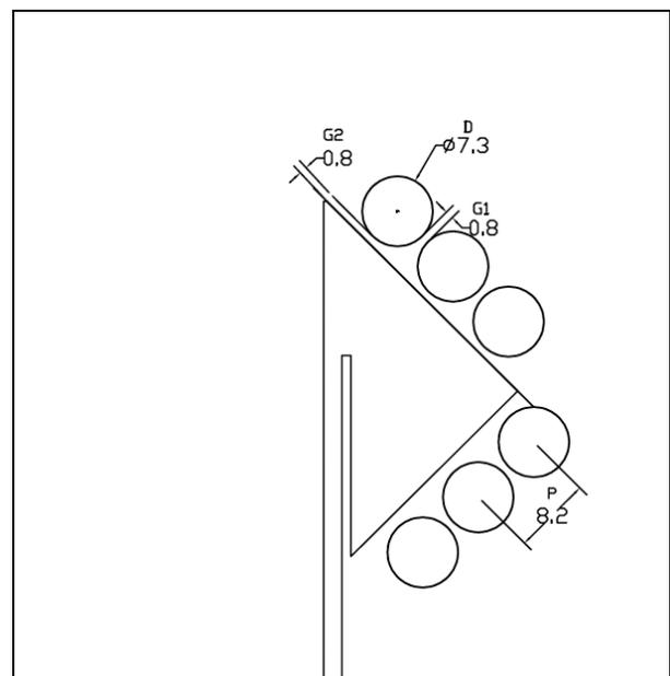
Figure 7: Numerical parameters of HMA with EBG (all dimensions are in mm)
