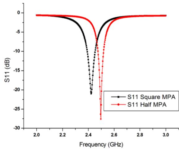
Figure 5: Simulated return loss for square microstrip antenna and Half Microstrip antenna
