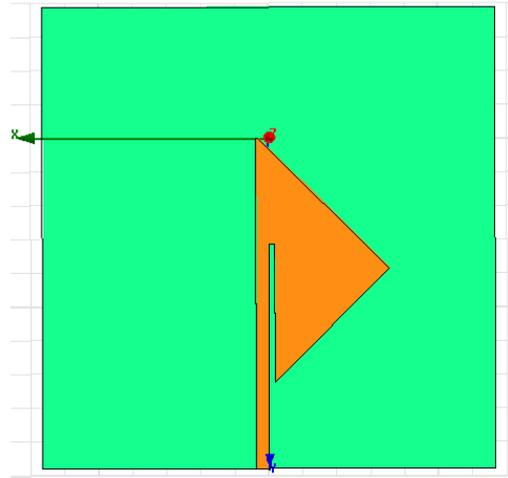
Figure 4: Simulation Model of Half microstrip antenna (HMA)
