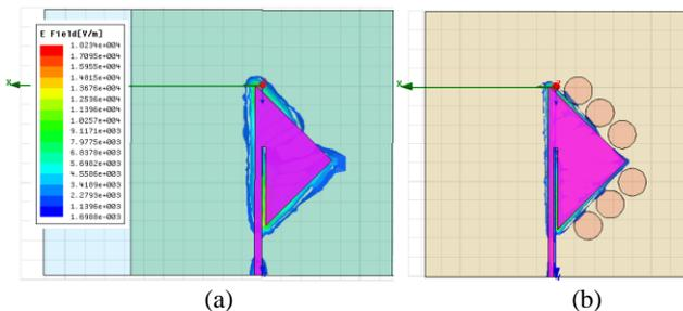
Figure 9: E-Field distribution of (a) HMA without circular EBG & (b) HMA with circular EBG
