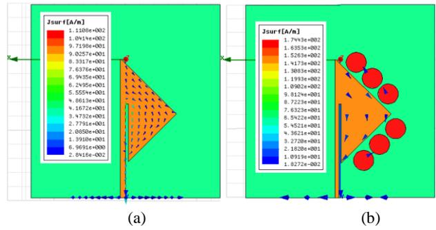
Figure 10: Current distribution of (a) HMA without circular EBG & (b) HMA with circular EBG
