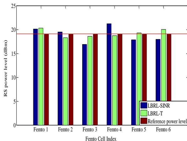
Figure 7: RS Power allocation for 6 Femto cells that underlay Macro cell with high load
