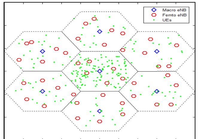
Figure 3: System topology of dense LTE-A HetNet
