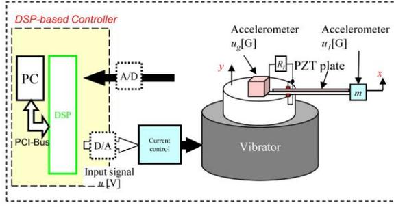
Figure 5: Experimental configuration for system identification experiment
