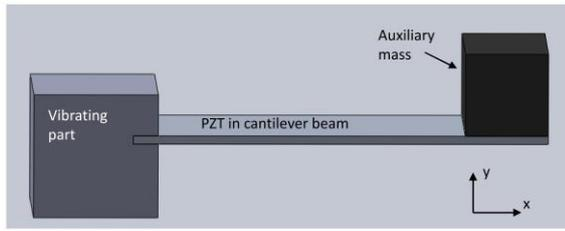
Figure 1: Typical structure of cantilever beam
