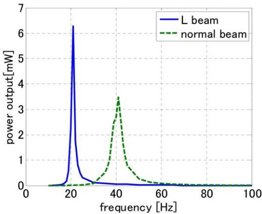
Figure 11: Output power of L-shape and typical cantilever beam piezoelectric power generator
