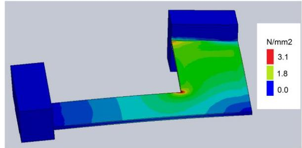
Figure 3: Stress distribution analysis of L-shape aluminum plate with Solidworks software
