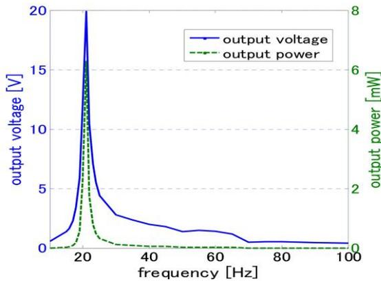
Figure 7: Frequency response of the power generator – peak voltage and power
