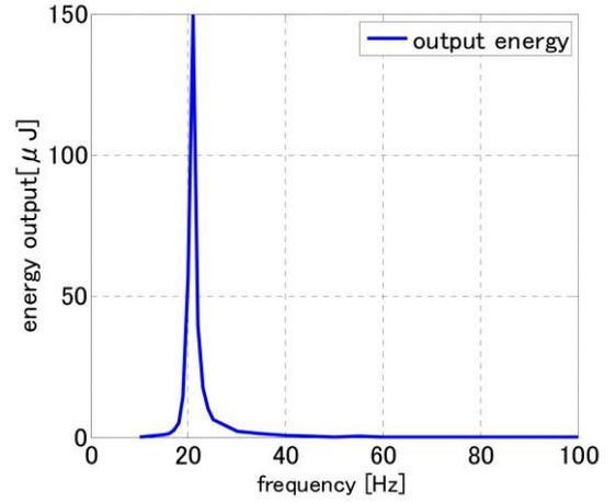
Figure 8: Frequency response of the power generator – peak energy for half cycle of output
