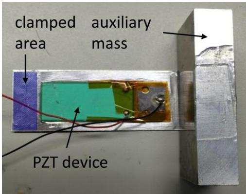
Figure 10: Typical cantilever beam with PZT device bonded on the top surface
