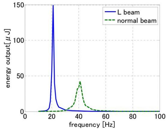
Figure 12: Output energy of L-shape and typical cantilever beam piezoelectric power generator
