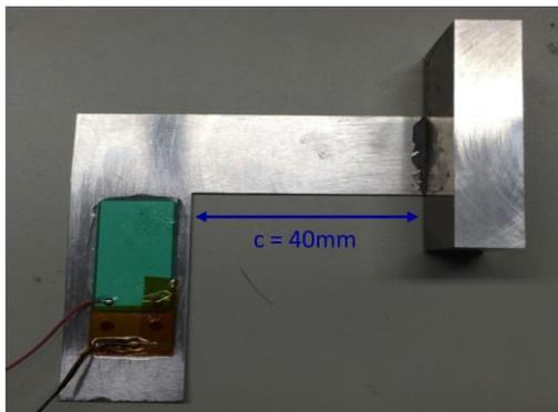
Figure 4: Prototype model of L-shape PZT power generator
