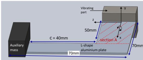
Figure 2: L-shape aluminum plate with auxiliary mass
